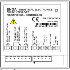
Logic output of the instrument is not electrically insulated from the internal circuits. Therefore, when using a grounding thermocouple, do not connect the logic output terminals to the ground.
