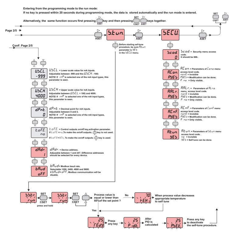
While holding  $\bigcap_{CSET}$  key, run message flashes. Then when  $\bigcap_{\triangle}$  key is pressed, self tune mode is entered if there is no probe failure. If process value is appropriate to begin self tune,  $rEd\mathcal{Y}$  message flashes. Then press any key to see P  $rd\mathcal{E}$ . message and self tune procedure begins.
